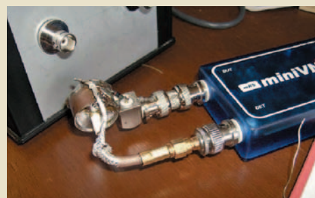
Fig. 32. Transformator – VNA meetopstelling.
