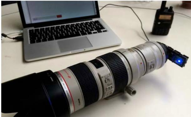
Yesterday I succeeded in hacking a 2006 design awarded Logitech Ultra Vision webcam to fit on my Canon EF 70-200mm EF USM II lens. With a 2x extender, the 1.3 MP 5mm sensor translates this camera in a huge 2800mm tele lens unit! This is needed to get a good view from the relay station to the iSémaphore, apx. 1km away.
